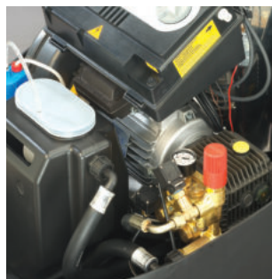
Rotary pump with ceramic plungers
